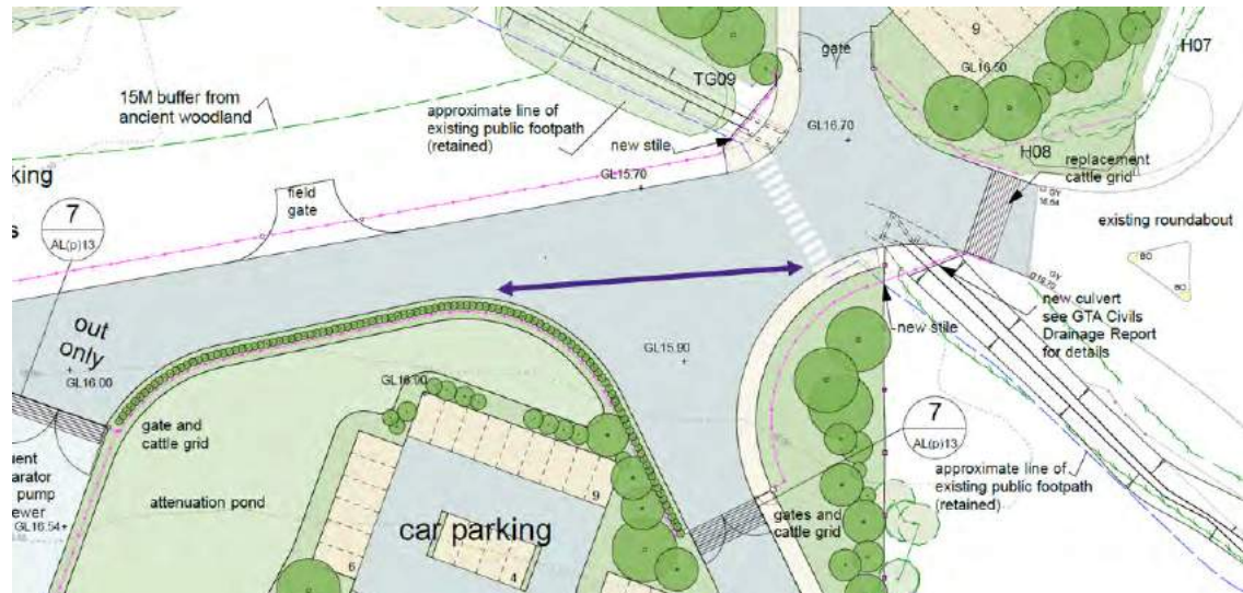
Figure 4: Pedestrian Desire Line Across the Eastern Access Junction to the Southern Part of the Site
